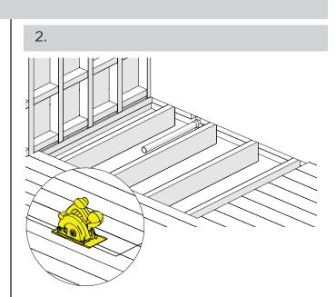
Carefully cut out the marked area on the floorboards with the Circular Saw. Be careful not to cut away at joist underneath. Ensure pipework is installed.
