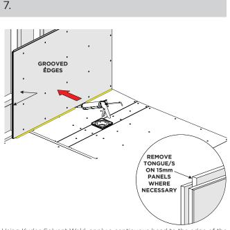
Using Kudos Solvent Weld, apply a continuous bead to the edge of the shower base, as shown.
