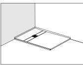
FLOOR & SKIRTING INSTALLATION Entire floor covered using the appropriate Aqua4ma panels. The walls are fitted with the Aqua4ma skirting panels.
