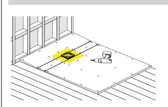
Secure the tray in place using drywall screws. Screw outside the parameters (indicated yellow) so that you miss the Square Steel Support Plate underneath (300mm x 300mm).
