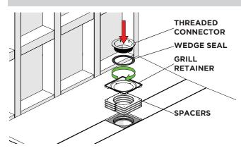
Place tray into position. Refer to Waste instructions to fit the Threaded Connector, Wedge seal, Grill Retainer and Height Spacer(s). Twist the Threaded connector into the Waste. This will tighten and secure tray to waste.
