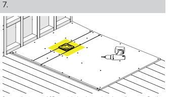
Secure the tray and 25mm strip in place using drywall screws. On the tray screw outside the parameters (indicated yellow) so that you miss the Square Steel Support Plate underneath (300mm x 300mm).
