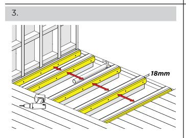
Cut down battens to suit space. Measure 18mm from the top of the joists and mark. Secure the battens in place using drywall screws, so that battens top surfaces are set 18mm below the joist top surface.
