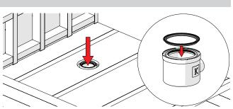
Connect waste body using 1½" / 42mm UK solvent weld waste pipe (not supplied), ensuring that the waste body is positioned to centre of the cut-out.
