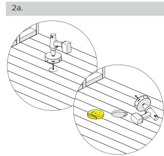
Remove the tray. In the centre of the marked position drill a hole with the Hole Saw 152mmOD, as shown. See section 2b. for solid floors.
