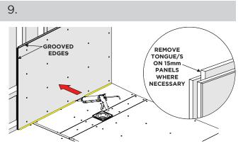
Using Kudos Solvent Weld, apply a continuous bead to the edge of the shower base, as shown.
