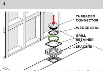
Place tray into position. Refer to Waste instructions to fit the Threaded Connector, Wedge seal, Grill Retainer and Height Spacer(s). Twist the Threaded connector into the Waste. This will tighten and secure tray to waste.
