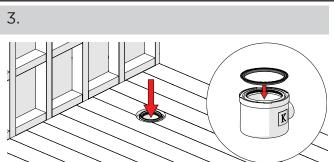
Connect waste body using 1%'' / 42mm UK solvent weld waste pipe (not supplied), ensuring that the waste body is positioned to centre of the cut-out.
