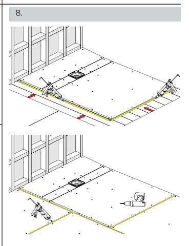
Using Kudos Solvent Weld, apply a continuous bead to the edge of the shower base, as shown.
