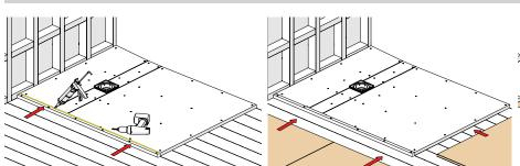
1. Using Kudos Solvent Weld, apply a continuous bead to the edge of the shower base, as shown where the 25mm strip is going. Lay the 25mm strip up to the edge of the base applying pressure to ensure the 25mm strip is fitted firmly against the base edge. Secure the 25mm strip in place using drywall screws (not supplied).
