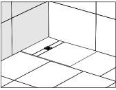
FULL INSTALLATION Entire floor and all walls are covered Entire walls within the shower area using the appropriate Aqua4ma panels.
